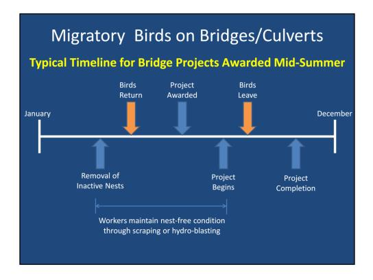
Typical scenario for dealing with birds on bridges. For LPA, local forces can remove existing nests during the INACTIVE season and monitor twice a week during active season (generally April 1 to July 31) to scrape off any nests being rebuilt. Schedules can be adjusted to get that work under contract. Another option, when you know you have an issue early in the project development phase, is to attempt to schedule bridge deck work (demo or deck removal or painting, etc) outside active season.
