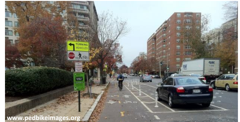
Figure 15: On-street parking establishes a physical barrier between the bike lane and motor vehicle lanes
